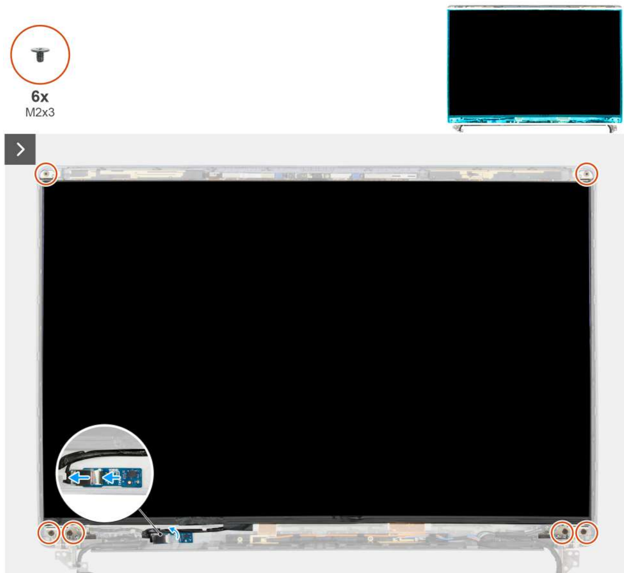
Figure 95. Removing the display panel
