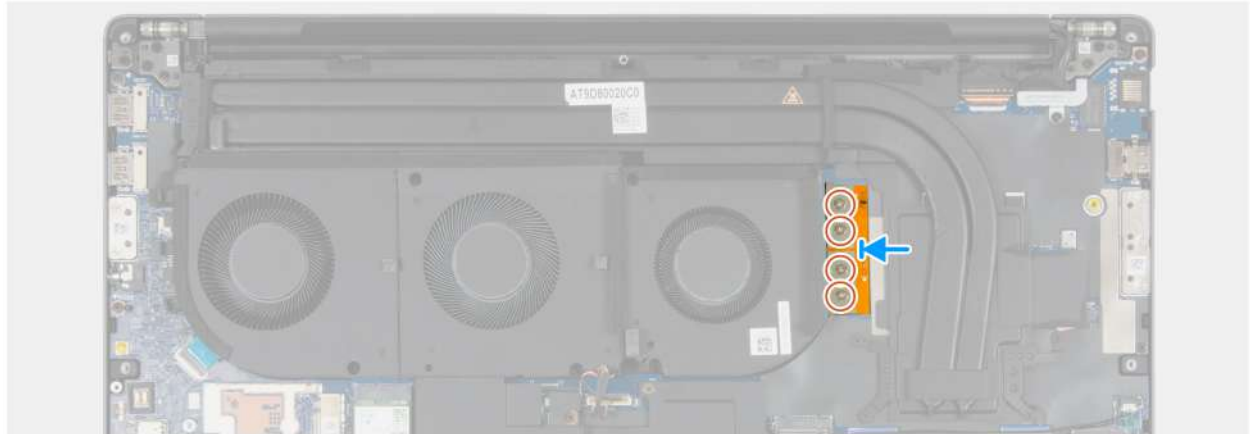
Figure 58. Installing the integrated FPC beam connector
