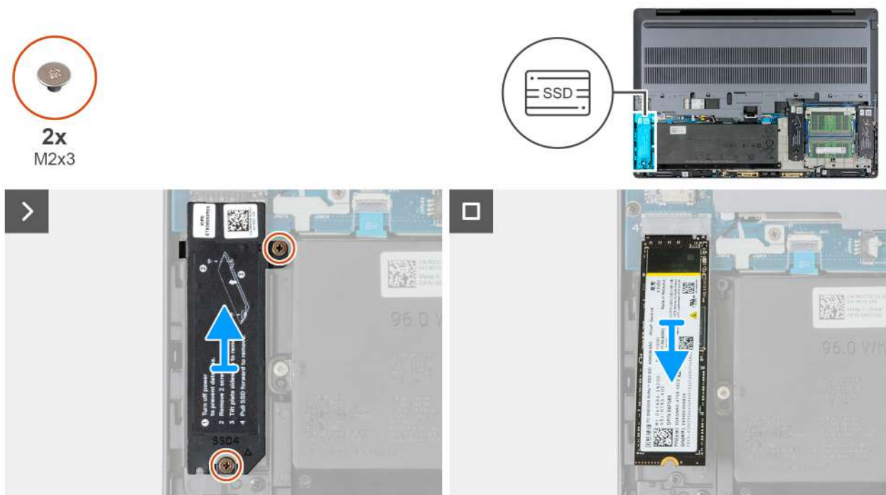
Figure 40. Removing the M.2 2280 SSD from slot 4 (SSD4)
