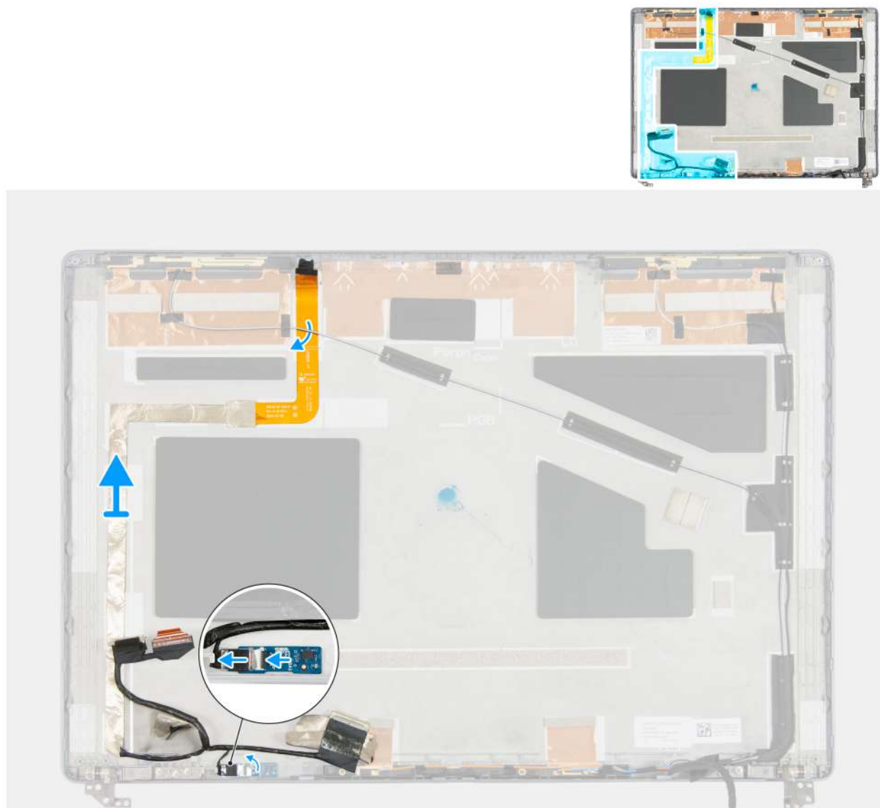
Figure 104. Removing the display cable
