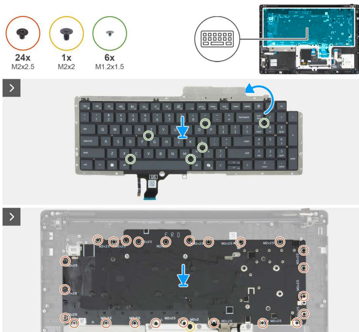
Figure 121. Installing the keyboard
