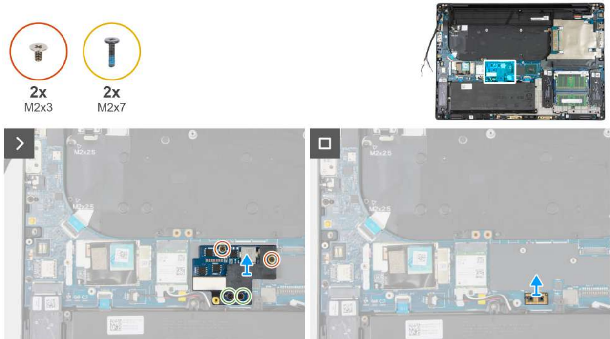
Figure 71. Removing the power board
