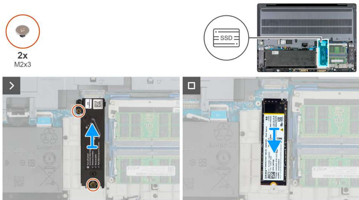
Figure 38. Removing the M.2 2280 SSD from slot 2 (SSD2)
