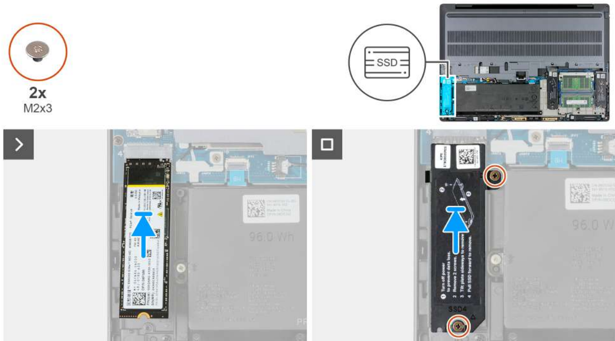
Figure 41. Installing the M.2 2280 SSD in slot 4 (SSD4)
