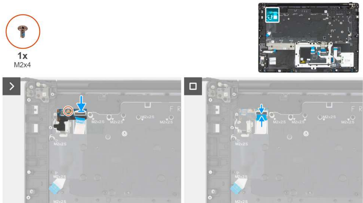
Figure 128. Installing the power button board
