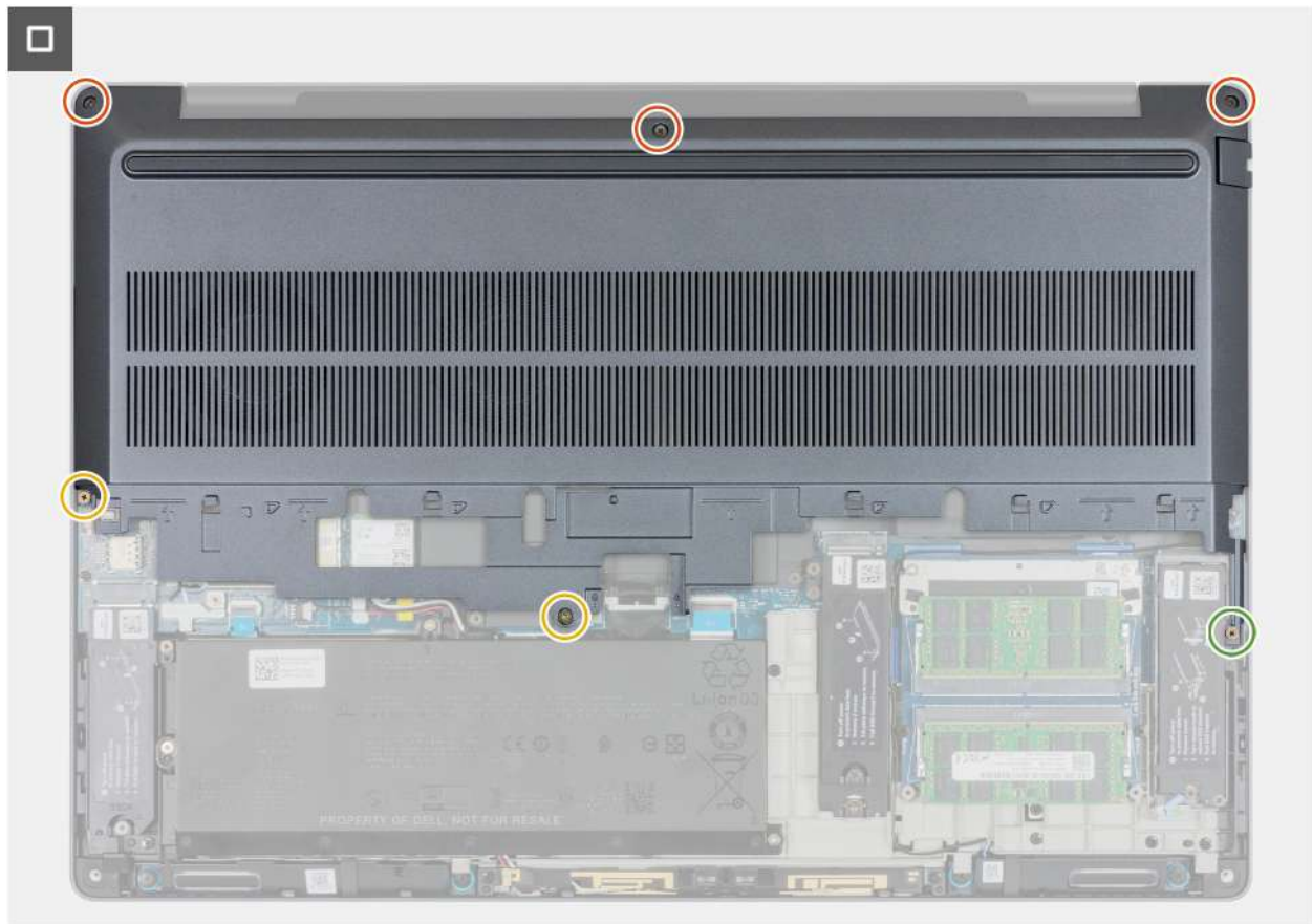
Figure 23. Tightening the three captive screws and replacing the three screws
