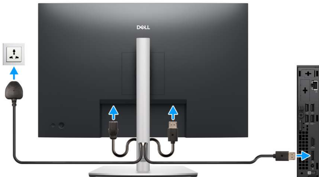
Figure 6. Connect the display
