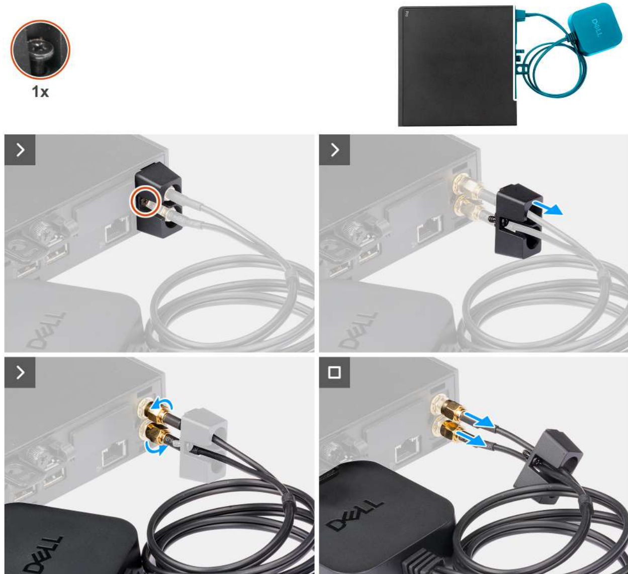
Figure 34. Removing external puck antenna
