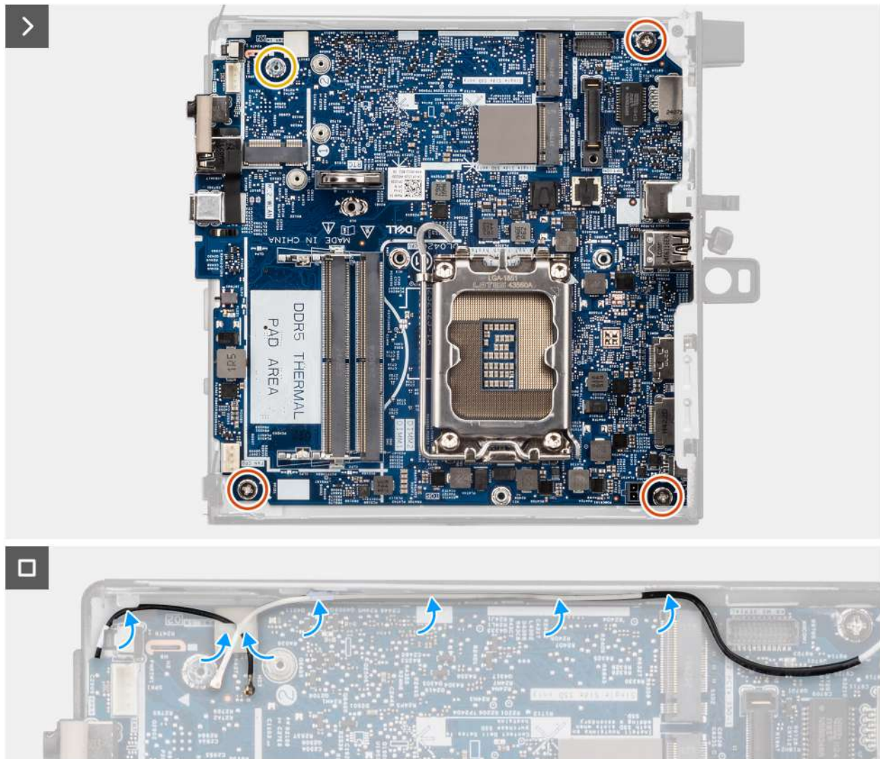
Figure 79. Installing the system board
