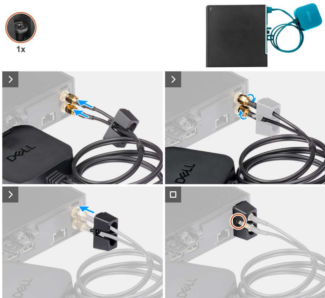
Figure 35. Installing external puck antenna
