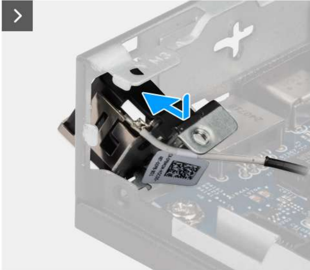
Figure 68. Installing the antenna module (white cable)
