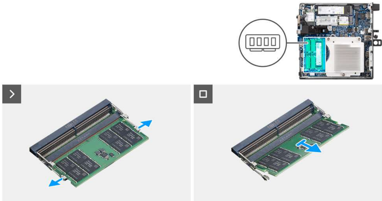
Figure 32. Removing the memory module
