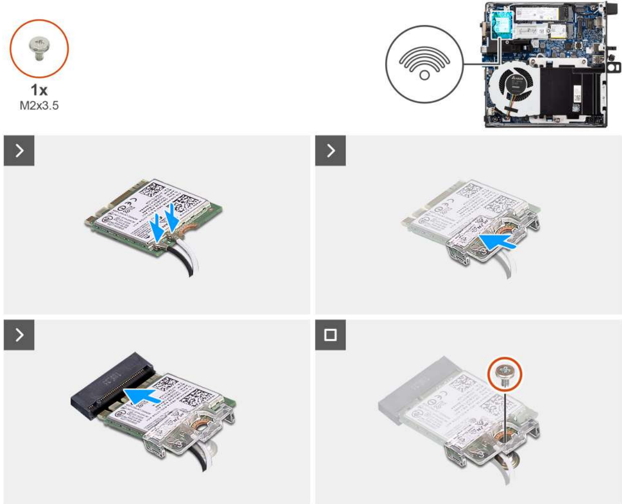
Figure 27. Installing the wireless card
