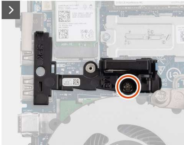
Figure 72. Removing the speaker holder
