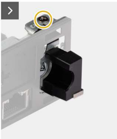
Figure 68. Installing the antenna module (white cable)
