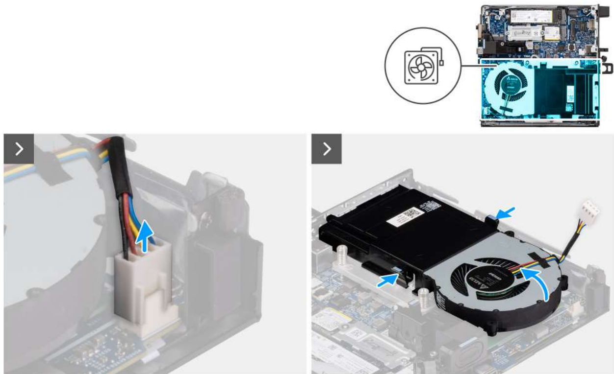
Figure 28. Removing the fan
