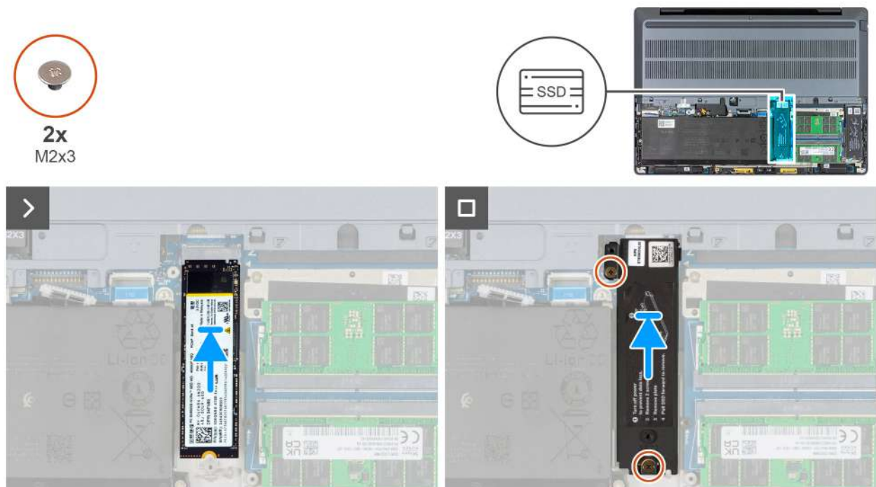
Figure 39. Installing the M.2 2280 SSD in slot 2 (SSD2)
