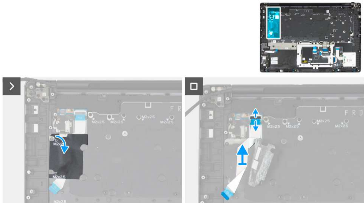
Figure 125. Removing the power button board cable
