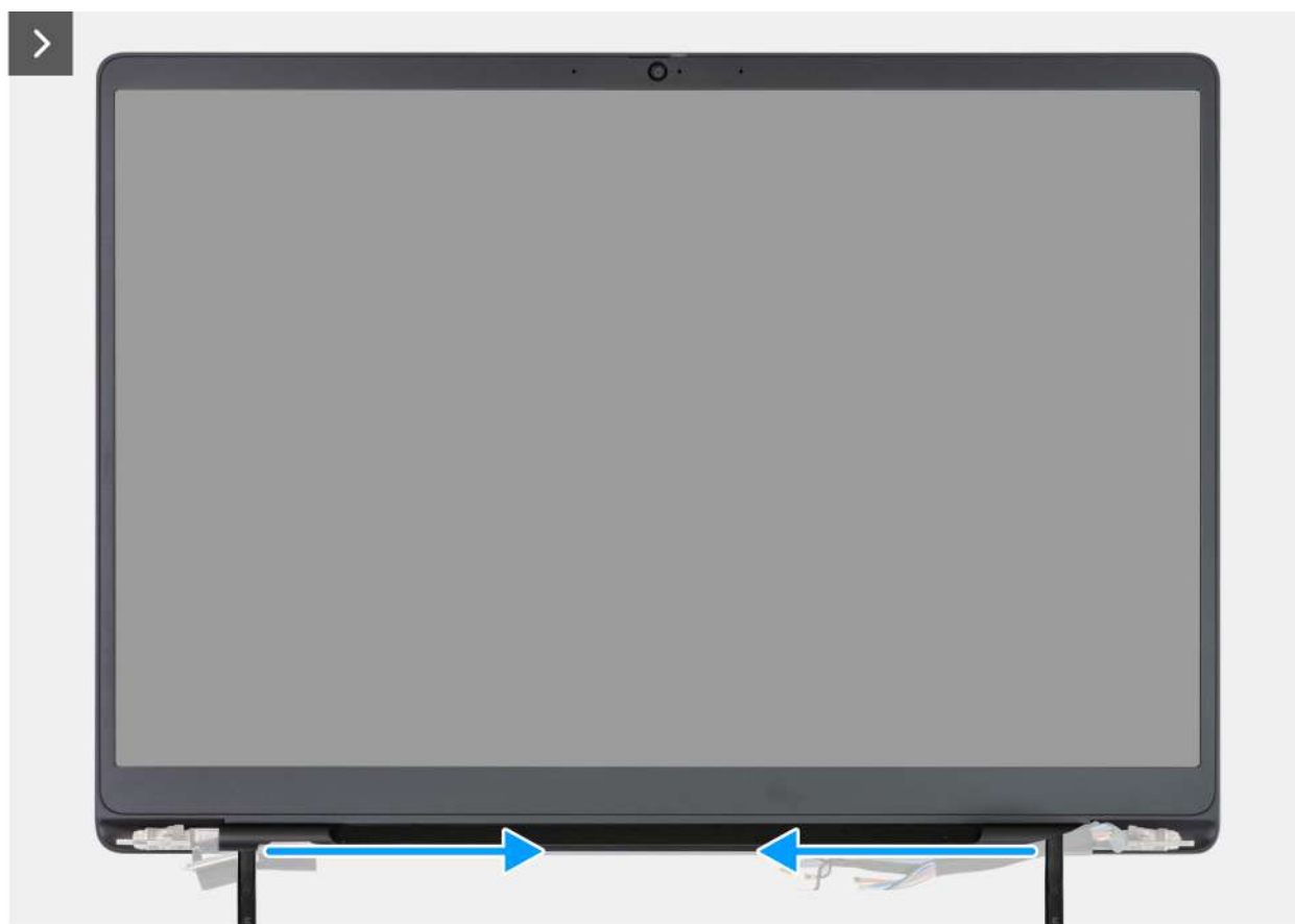
Figure 86. Removing the display bezel
