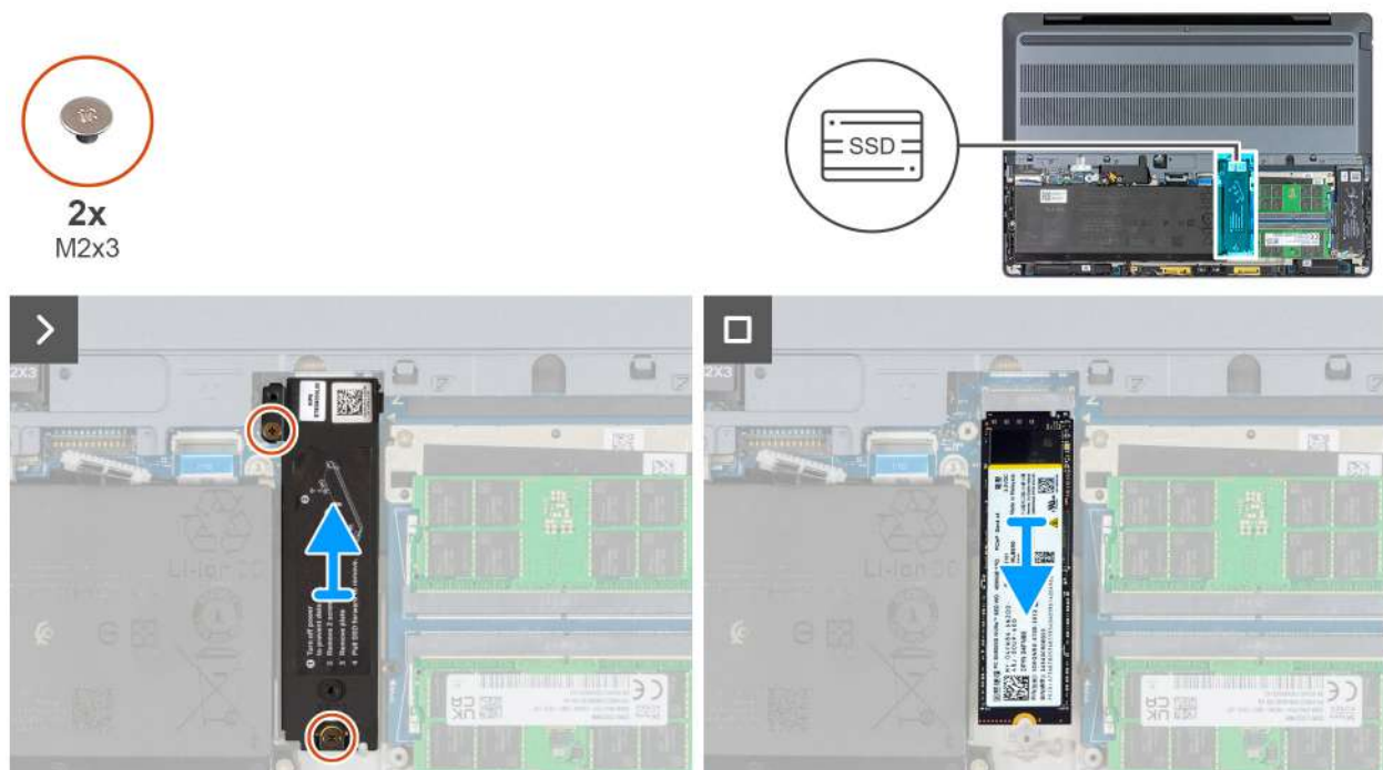
Figure 38. Removing the M.2 2280 SSD from slot 2 (SSD2)
