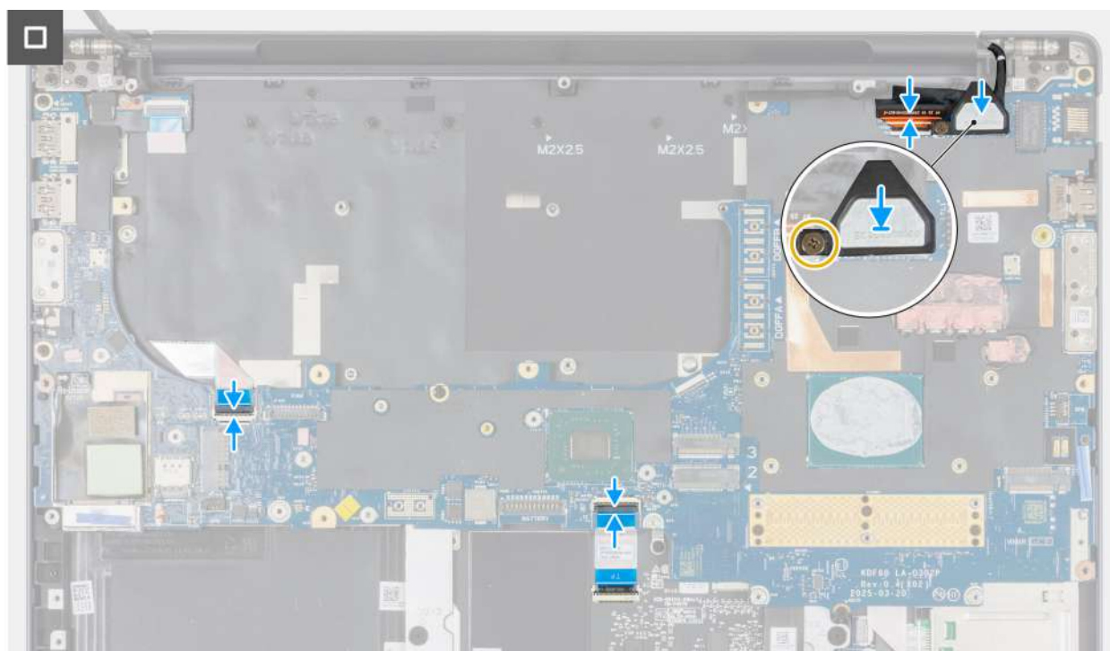
Figure 116. Installing the system board
