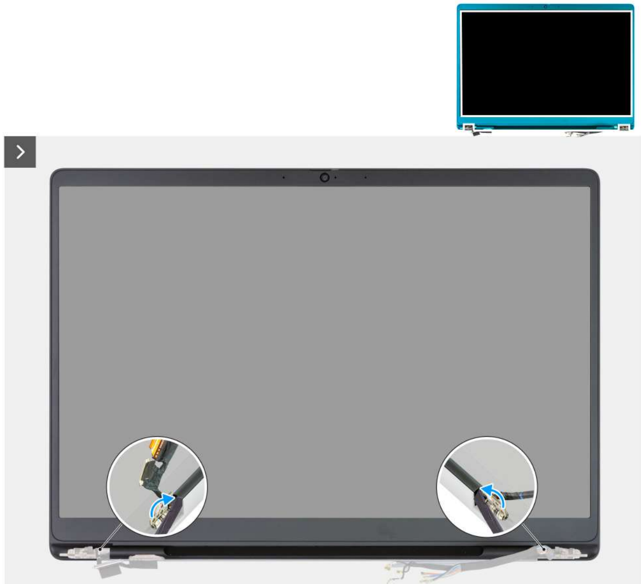
Figure 83. Removing the display bezel
