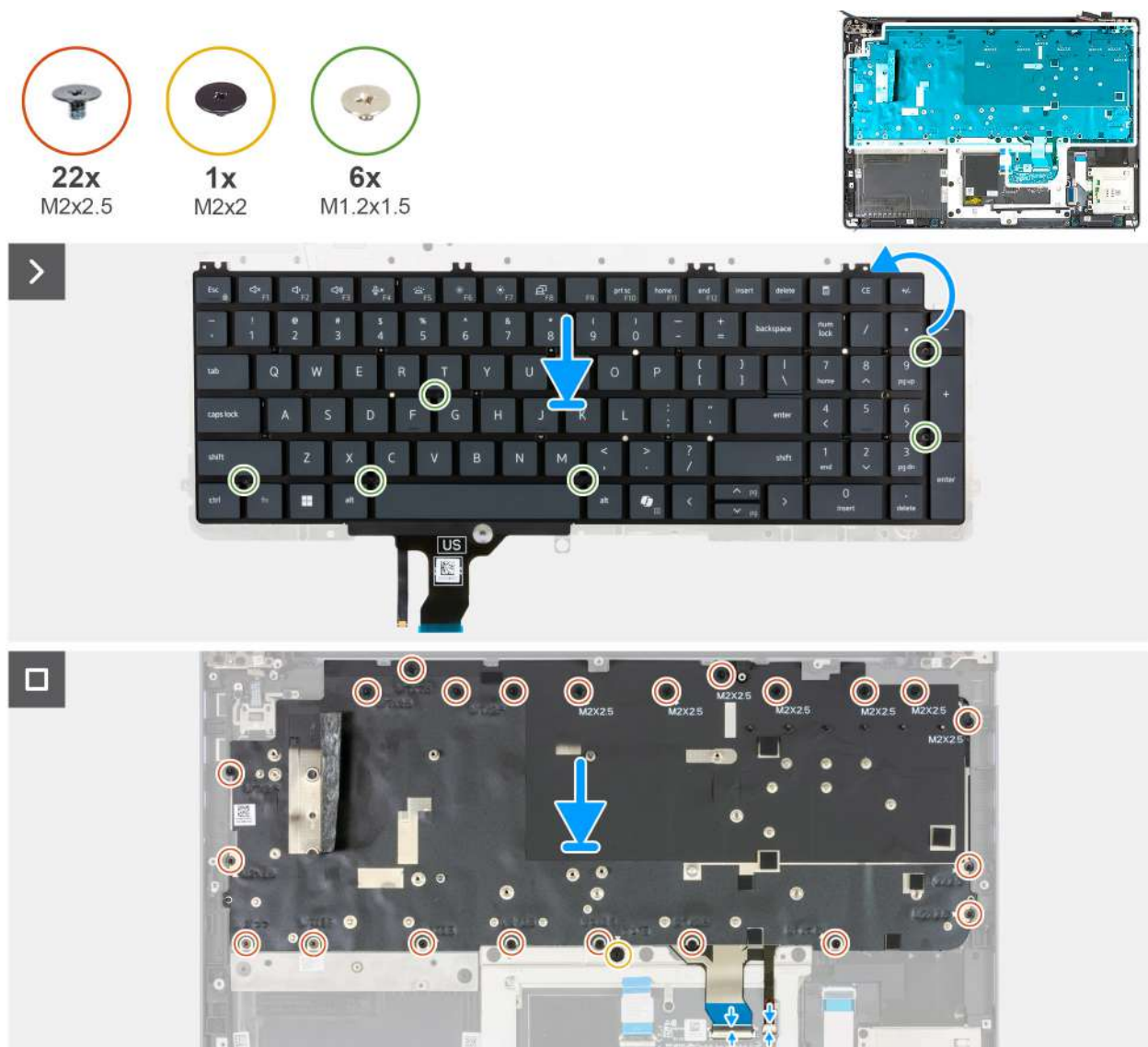
Figure 122. Installing the keyboard
