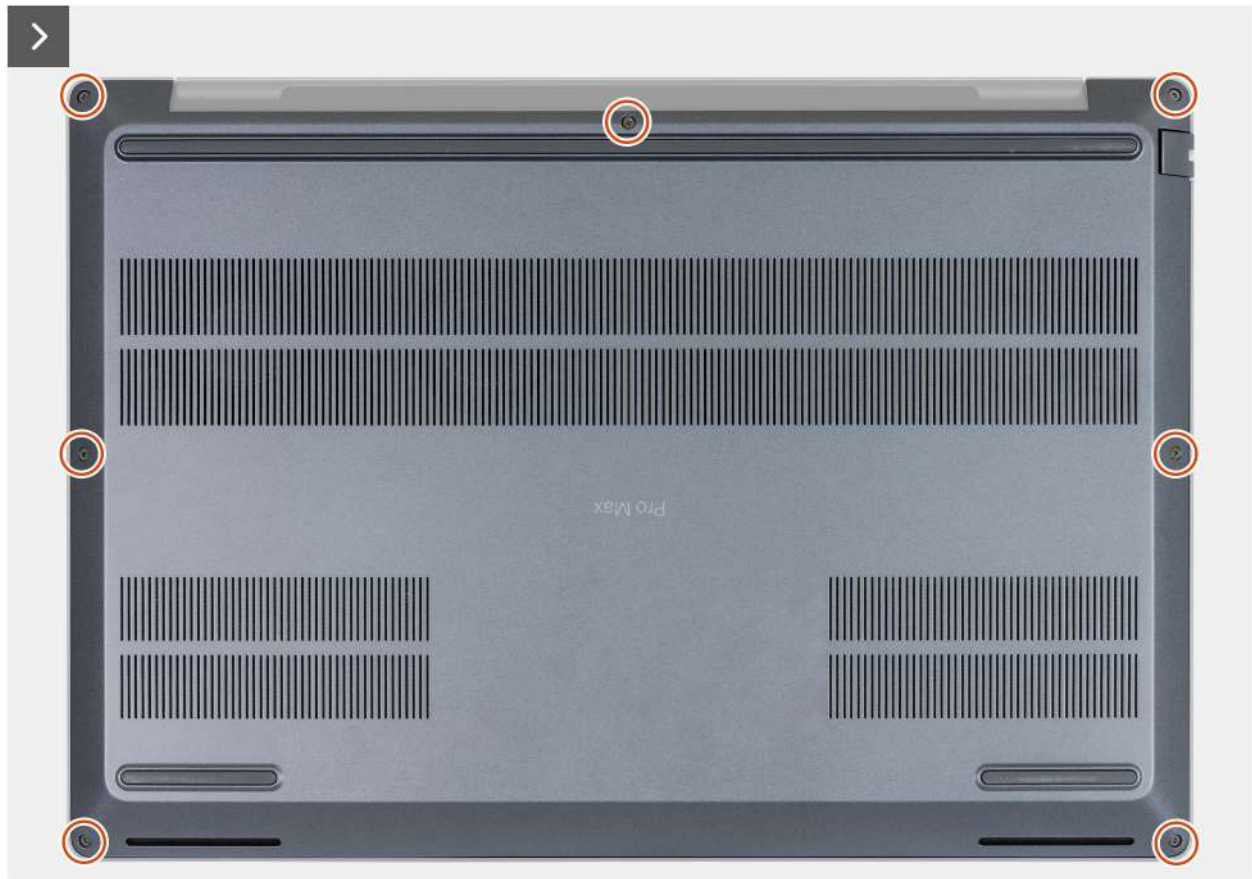
Figure 24. Loosening the captive screws
