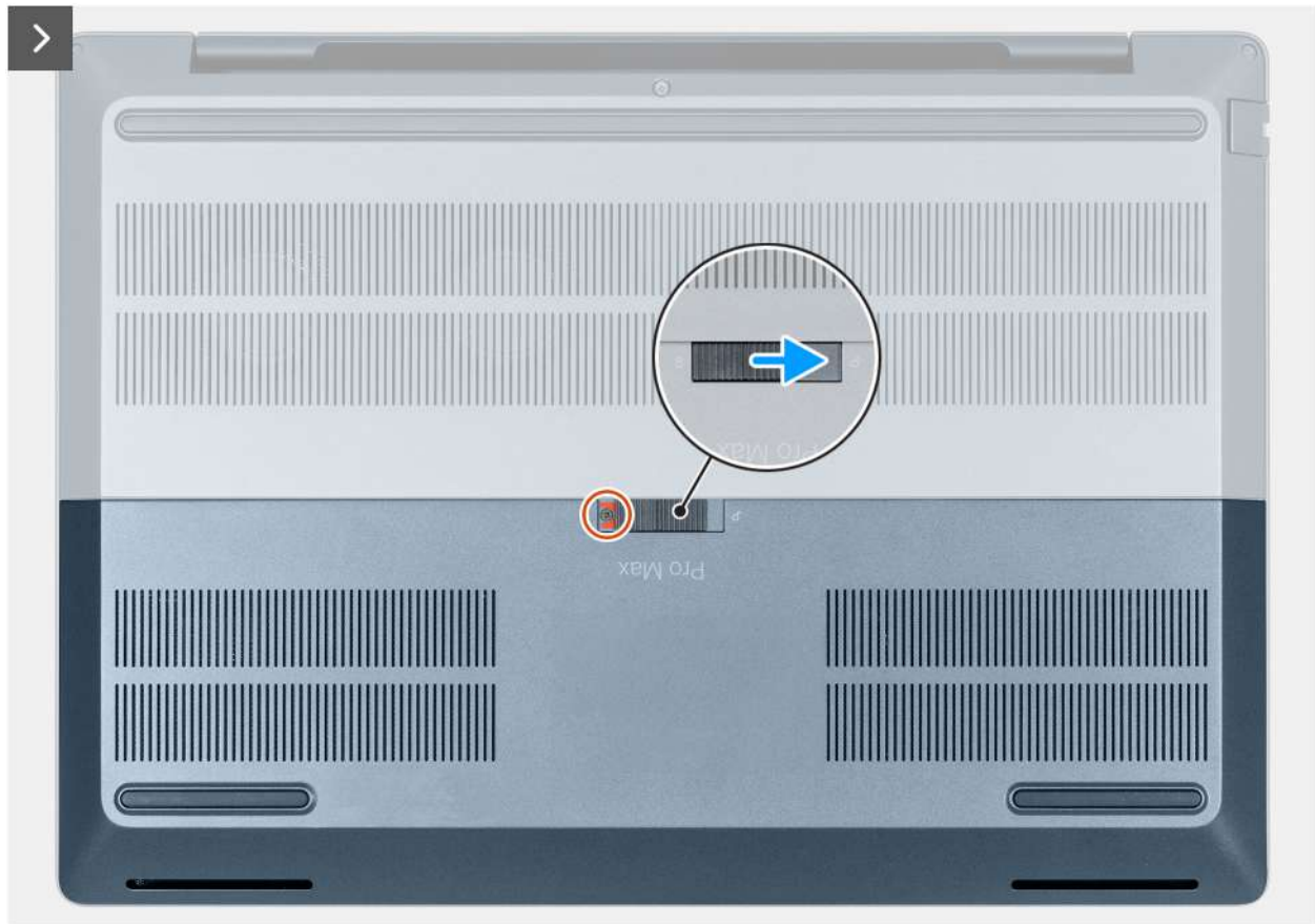
Figure 12. Sliding the door lock to the prelock position and removing the screw
