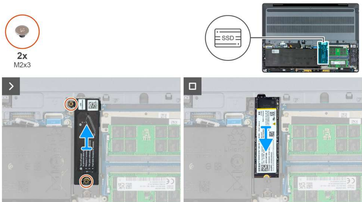
Figure 36. Removing the M.2 2280 SSD from slot 3 (SSD3)
