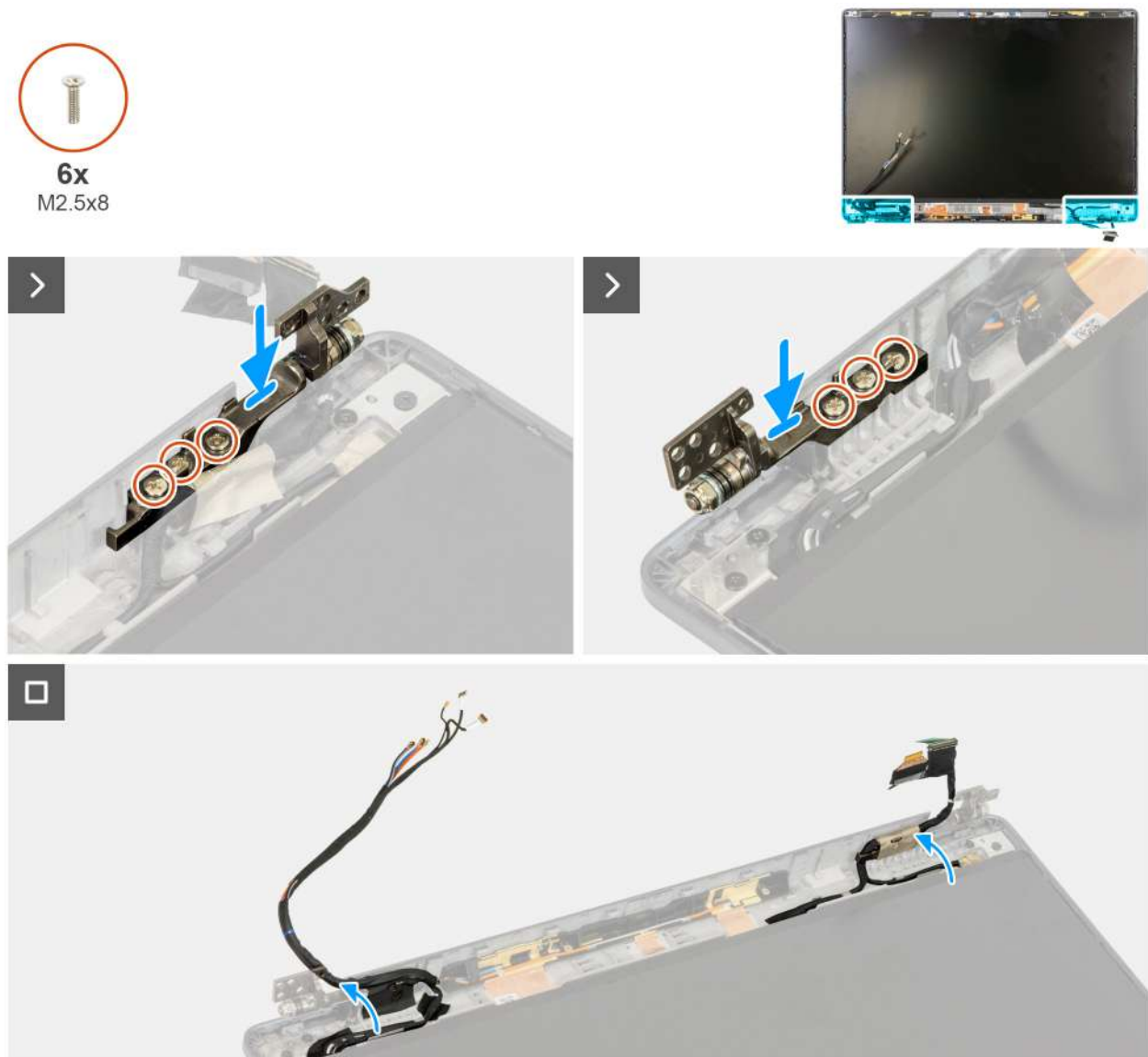
Figure 100. Installing the display hinges
