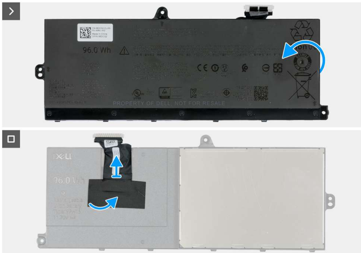
Figure 43. Removing the battery cable from the battery
