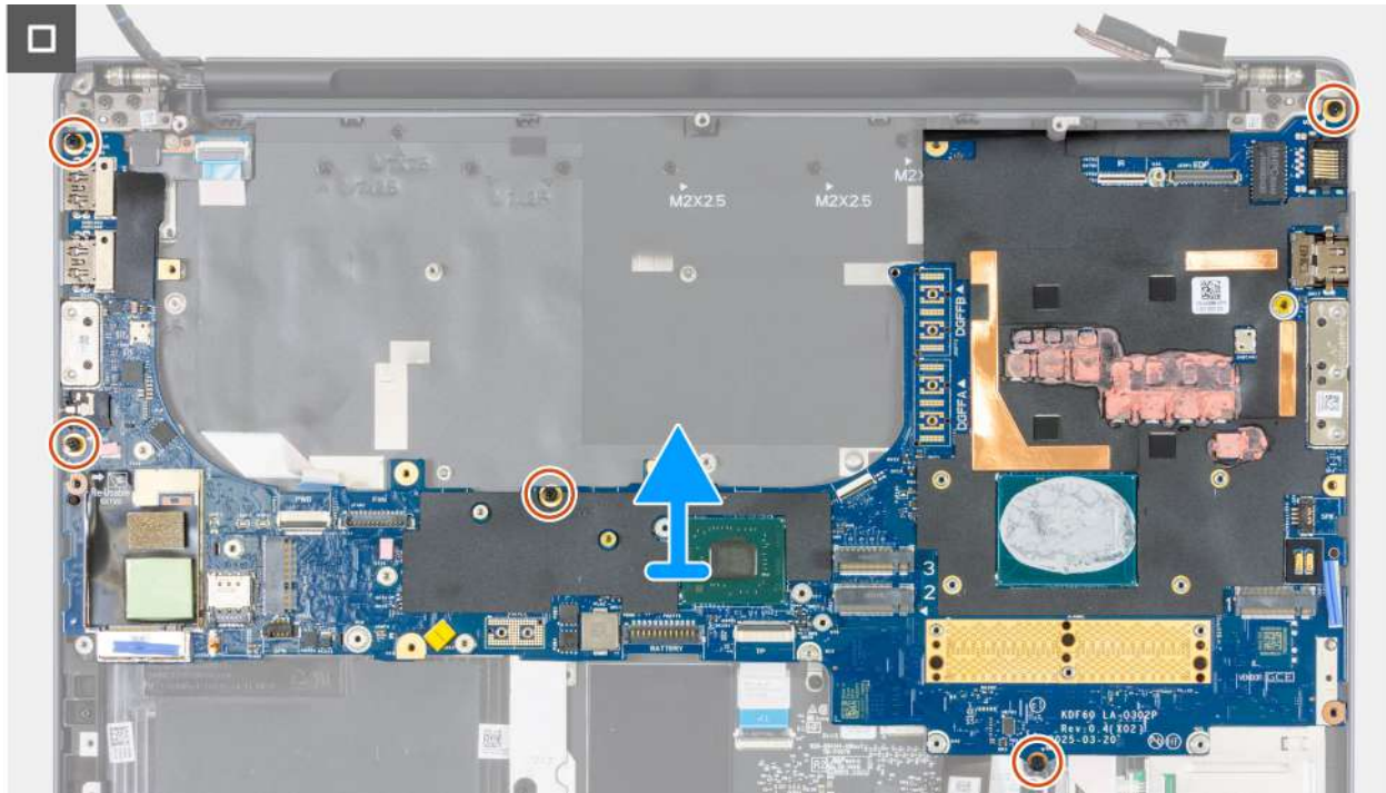
Figure 112. Removing the system board
