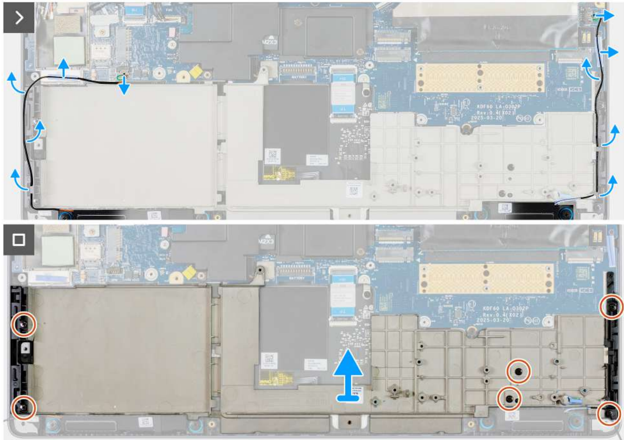
Figure 79. Removing the inner frame
