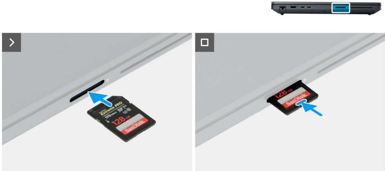
Figure 11. Installing the SD card
