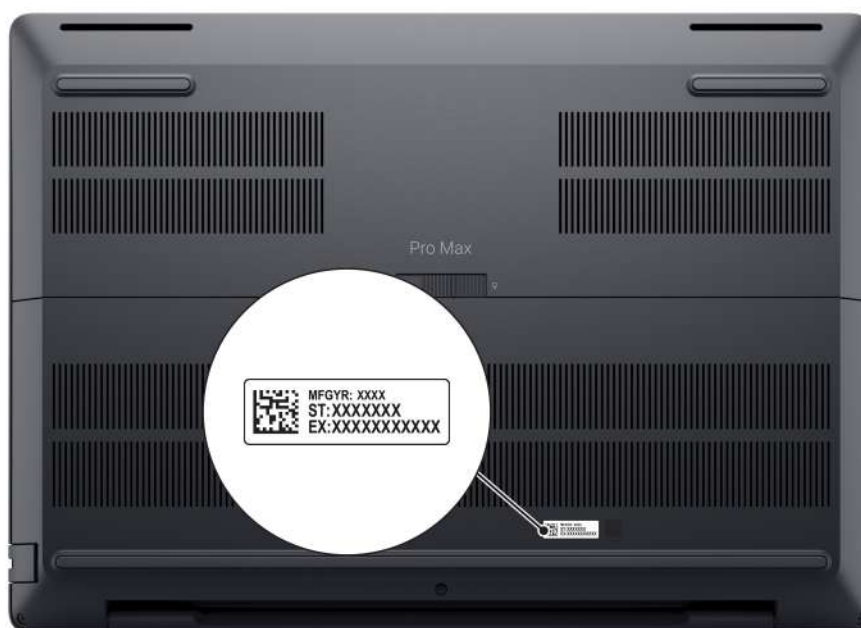
Figure 6. Service Tag/Express Service Code location
