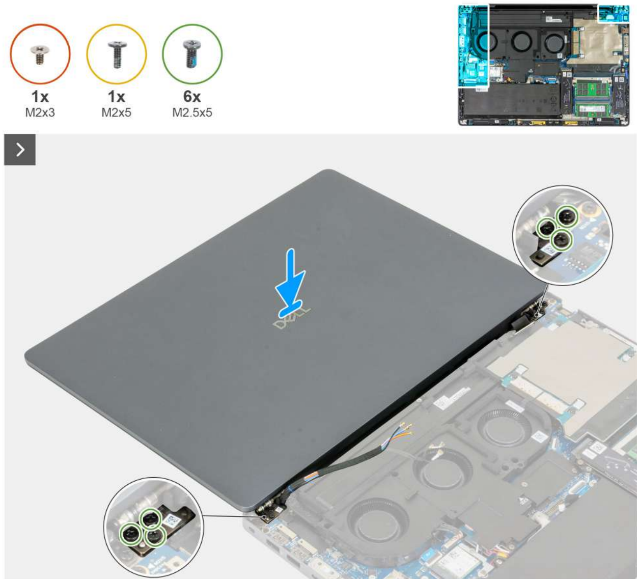
Figure 65. Installing the display assembly
