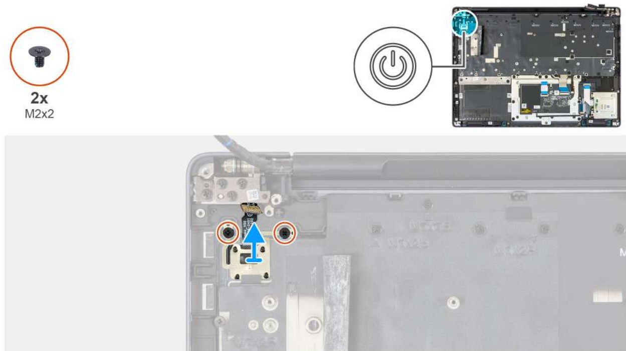
Figure 129. Removing the power button
