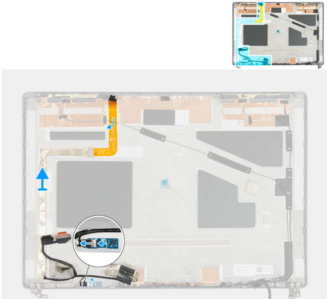
Figure 106. Removing the display cable
