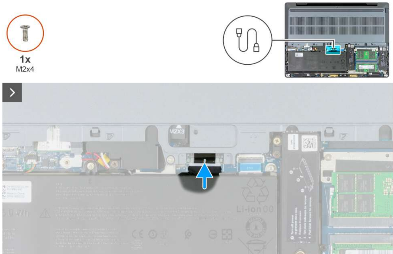
Figure 15. Connecting the battery cable
