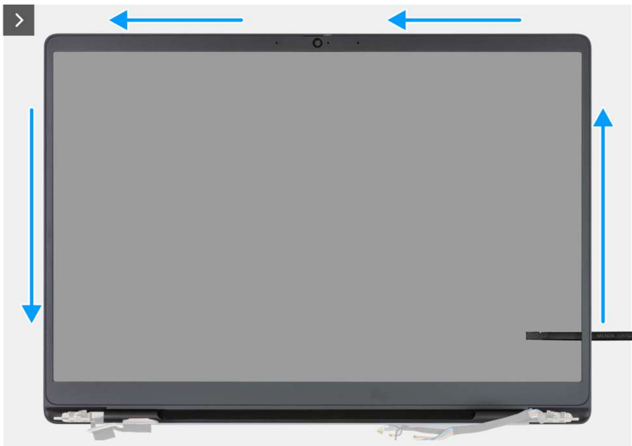
Figure 85. Removing the display bezel
