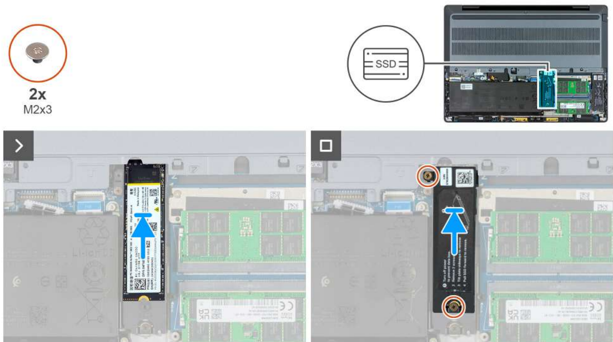
Figure 37. Installing the M.2 2280 SSD in slot 3 (SSD3)
