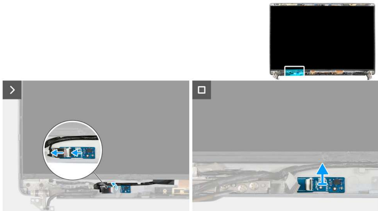
Figure 101. Removing the sensor board
