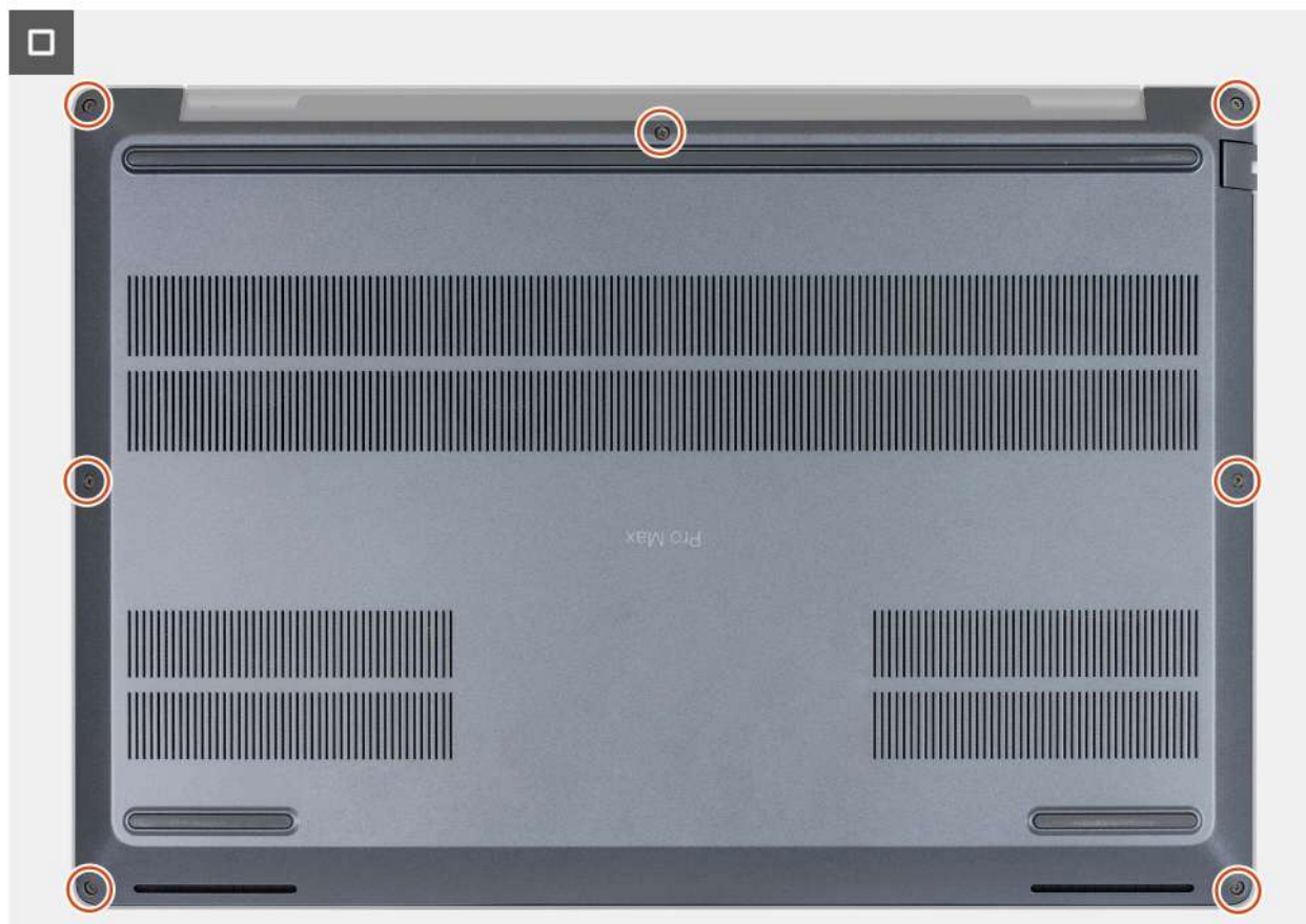
Figure 29. Tightening the captive screws
