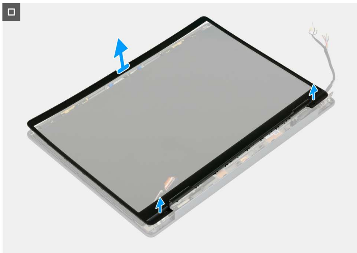
Figure 88. Removing the display bezel
