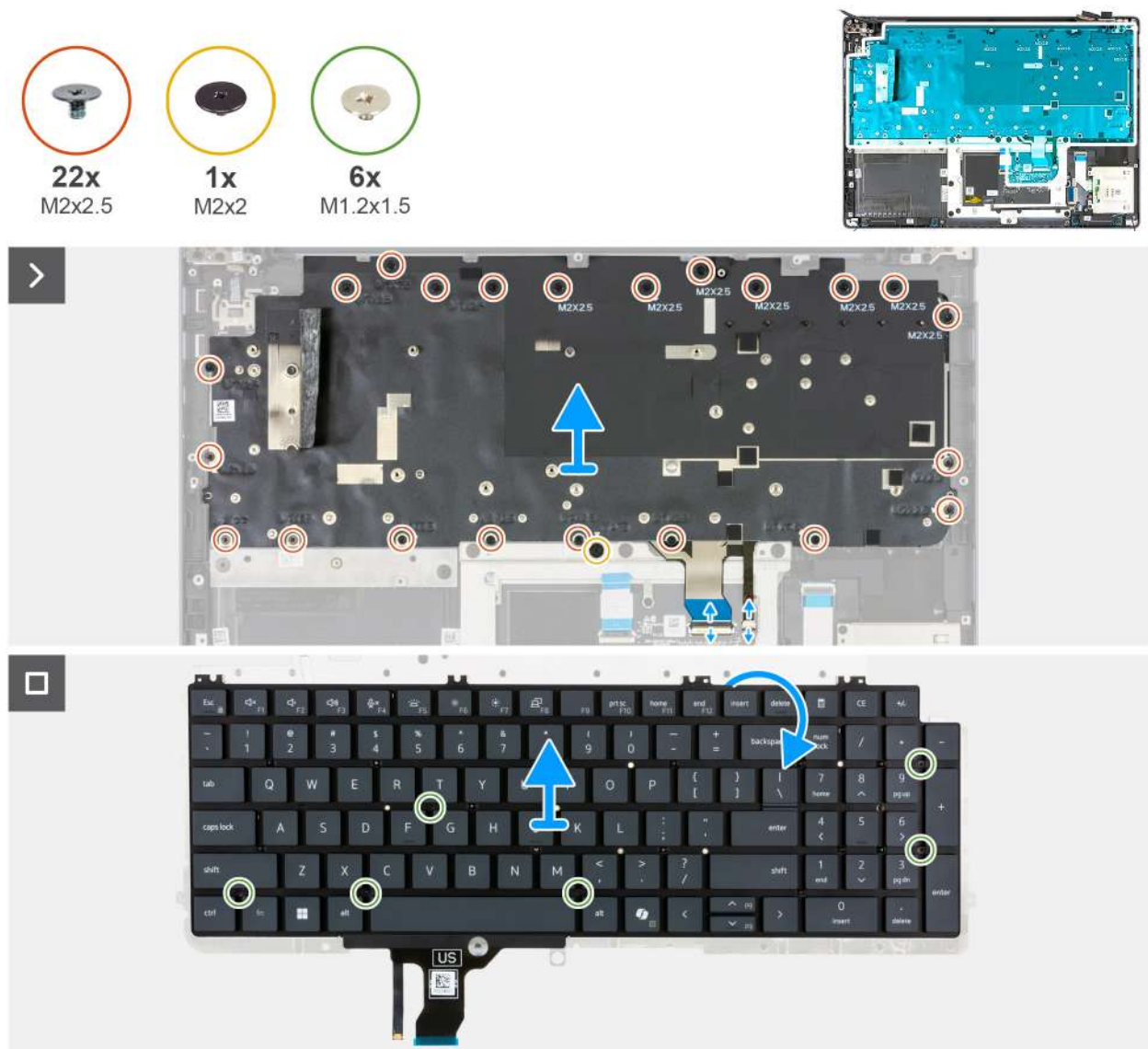
Figure 121. Removing the keyboard
