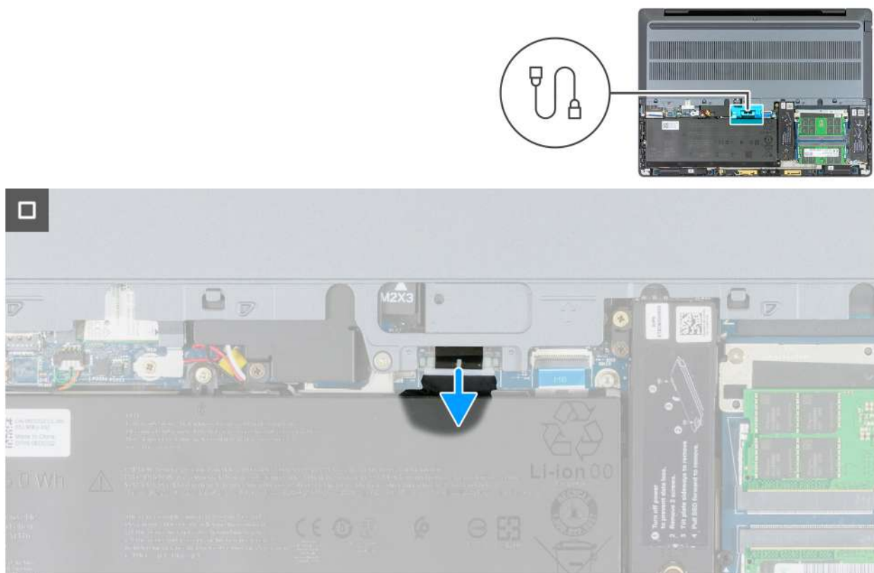
Figure 20. Disconnecting the battery cable
