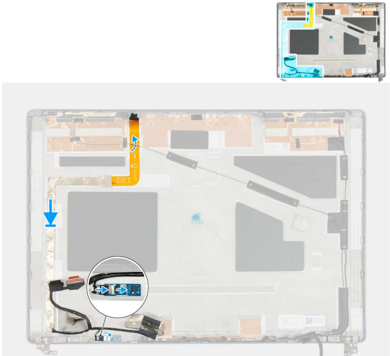
Figure 107. Installing the display cable
