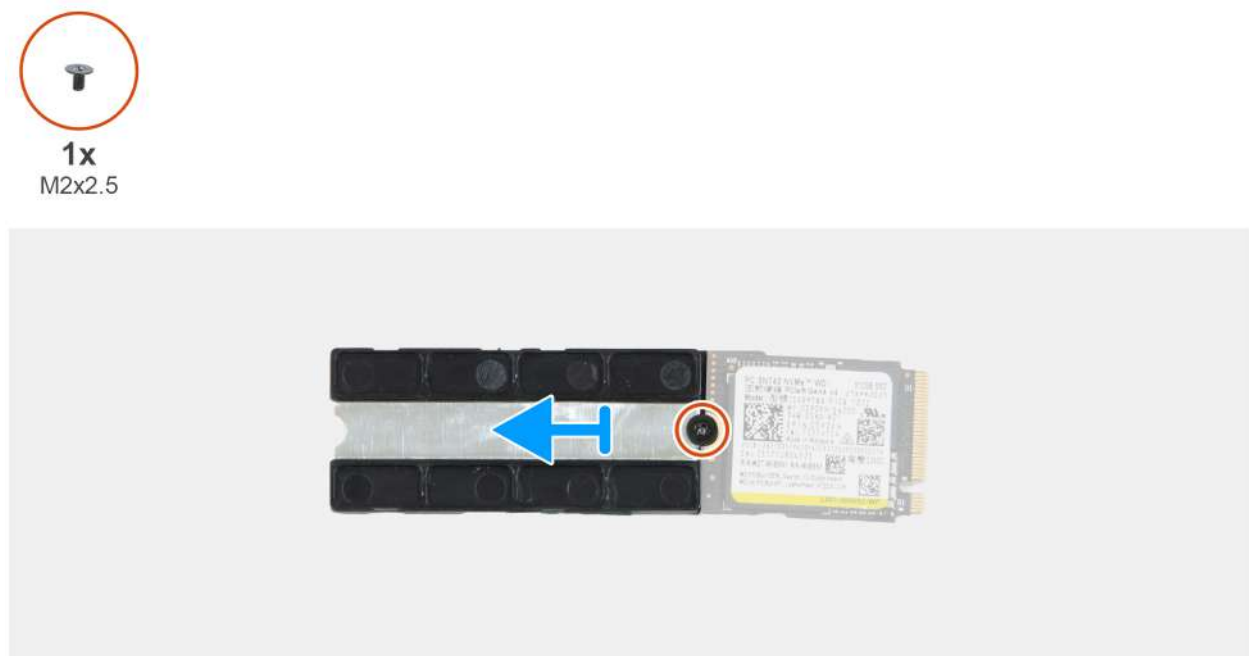
Figure 40. Removing the M.2 2230 SSD
