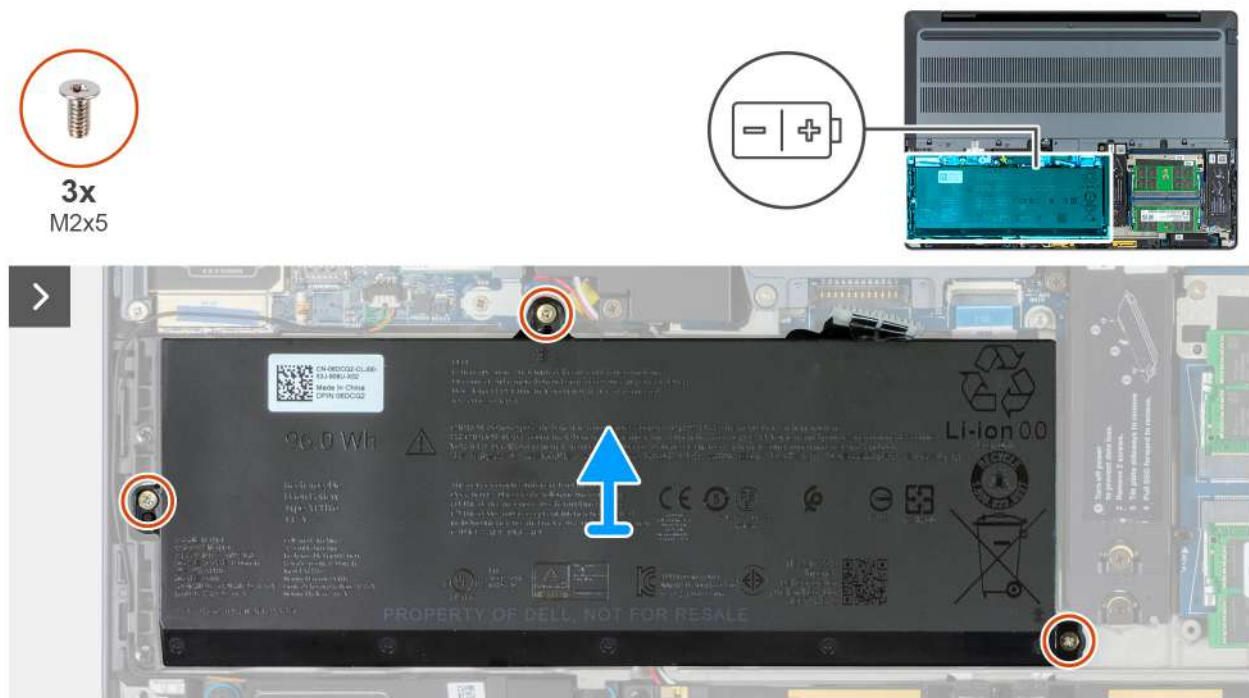
Figure 42. Removing the battery
