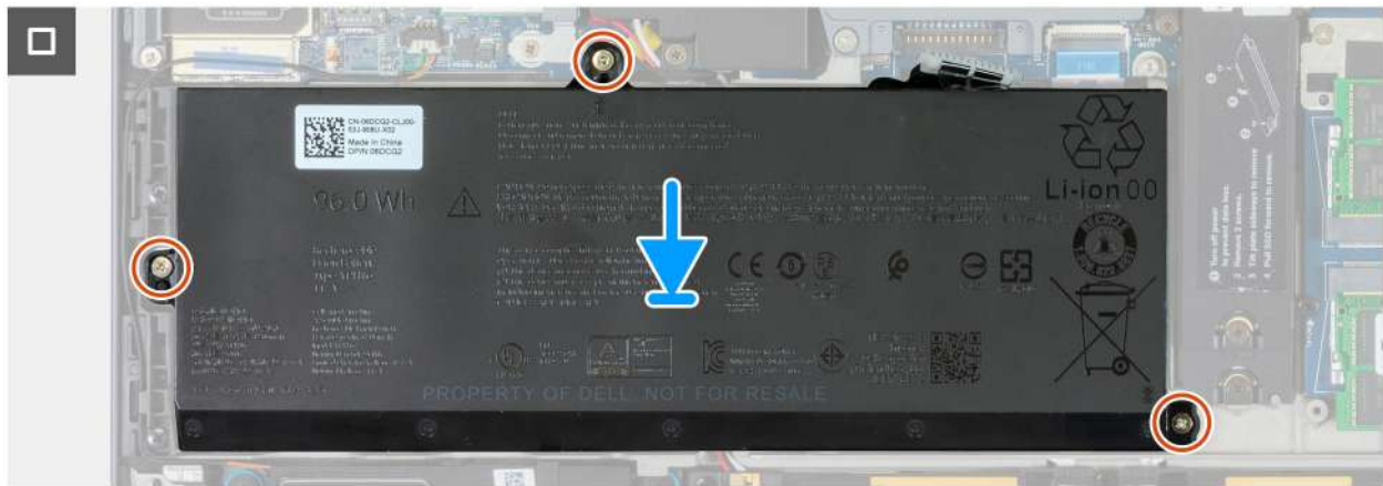
Figure 45. Replacing the battery
