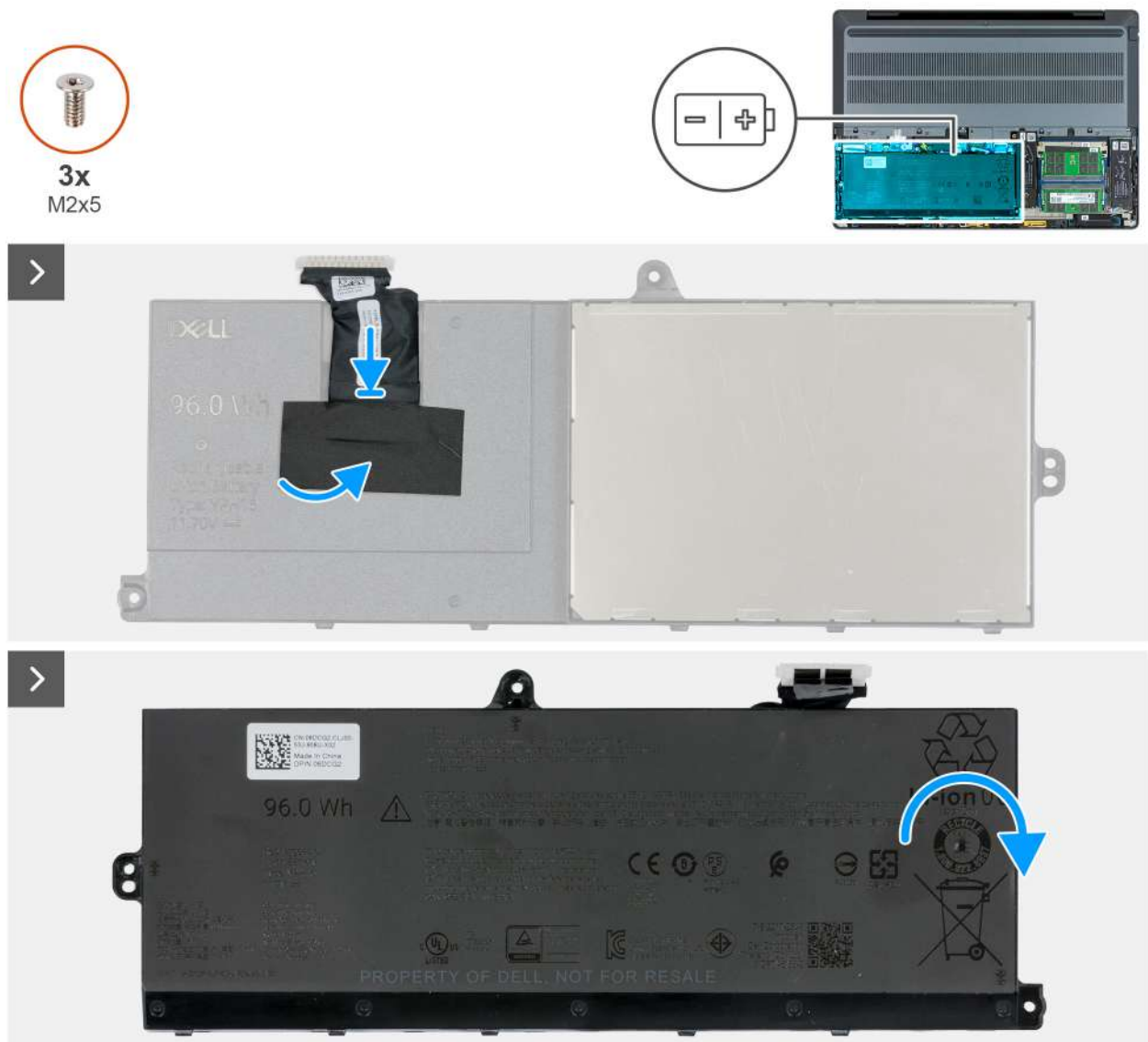
Figure 44. Replacing the battery cable
