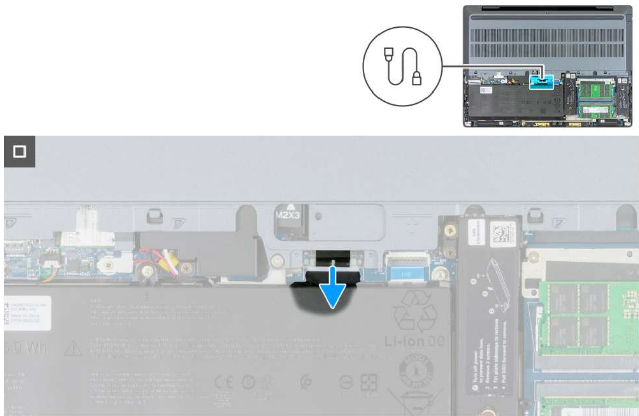
Figure 14. Disconnecting the battery cable
