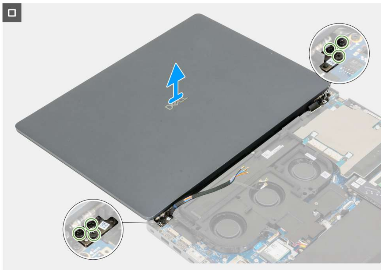
Figure 64. Removing the display assembly
