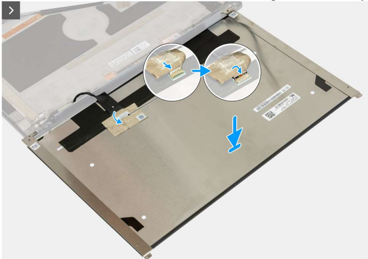
Figure 97. Installing the display panel for non-touchscreen displays
