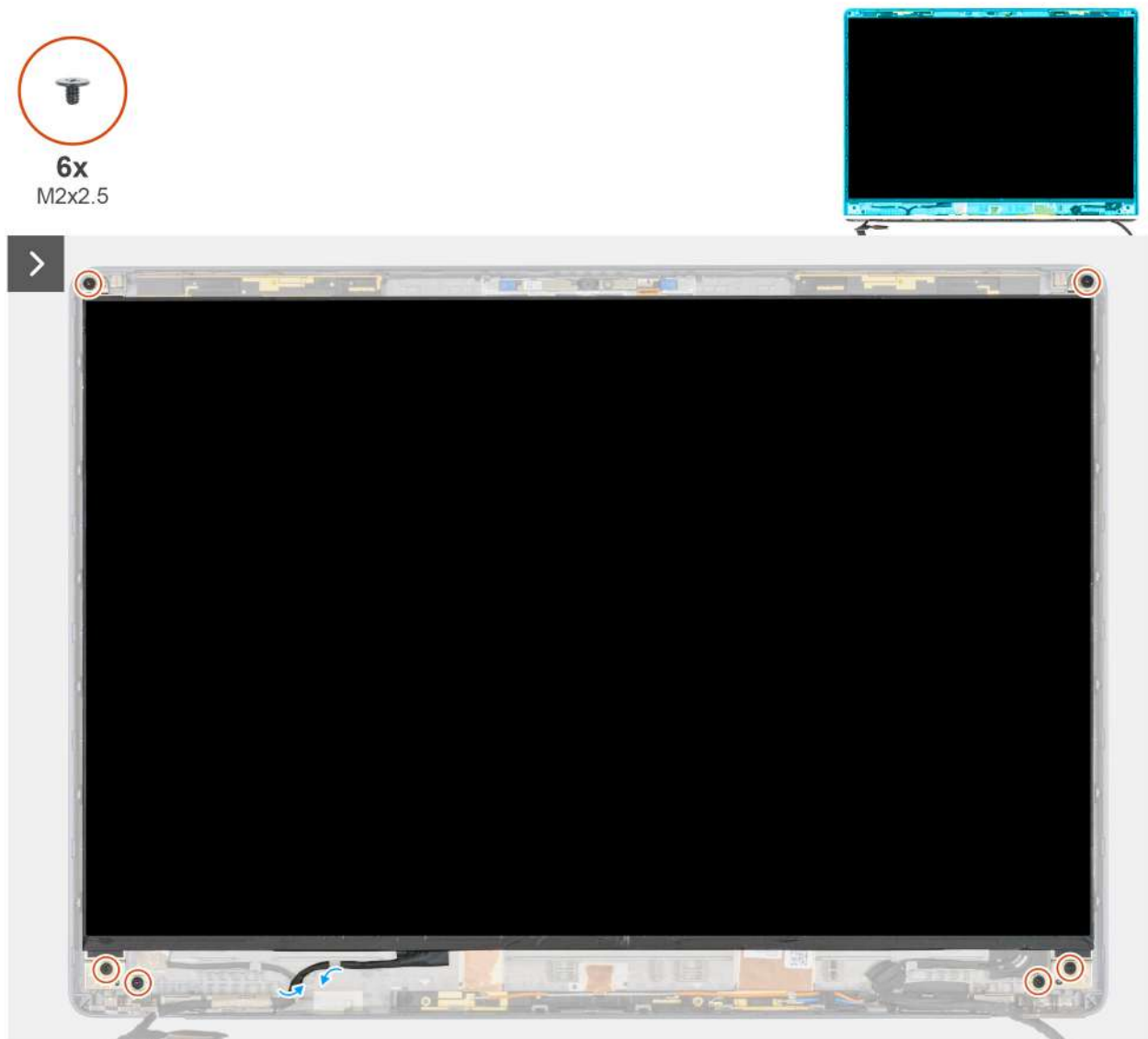
Figure 95. Removing the display panel for non-touchscreen displays
