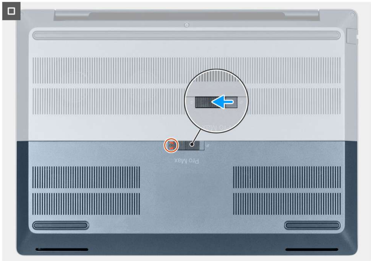
Figure 17. Replacing the screw and sliding the door lock to the lock position
