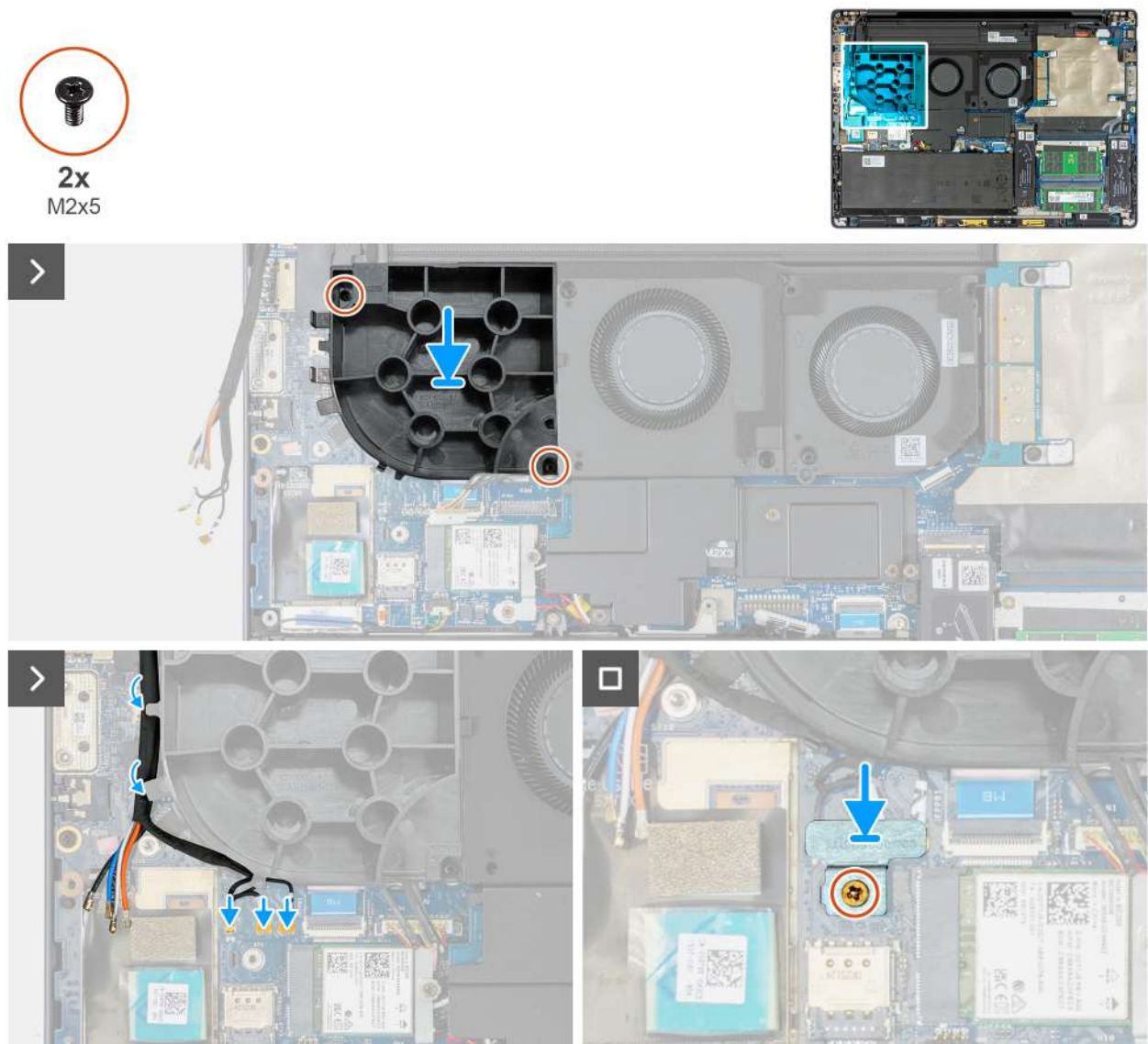
Figure 60. Installing the dummy fan
