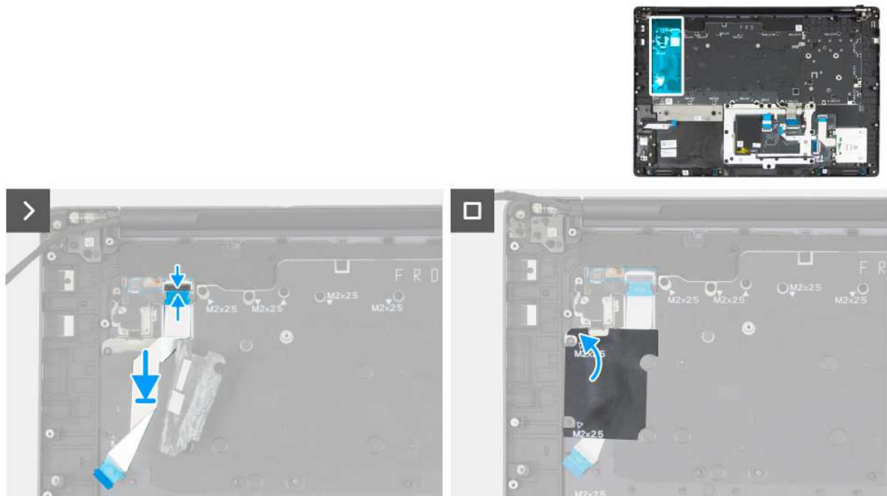
Figure 126. Installing the power button board cable
