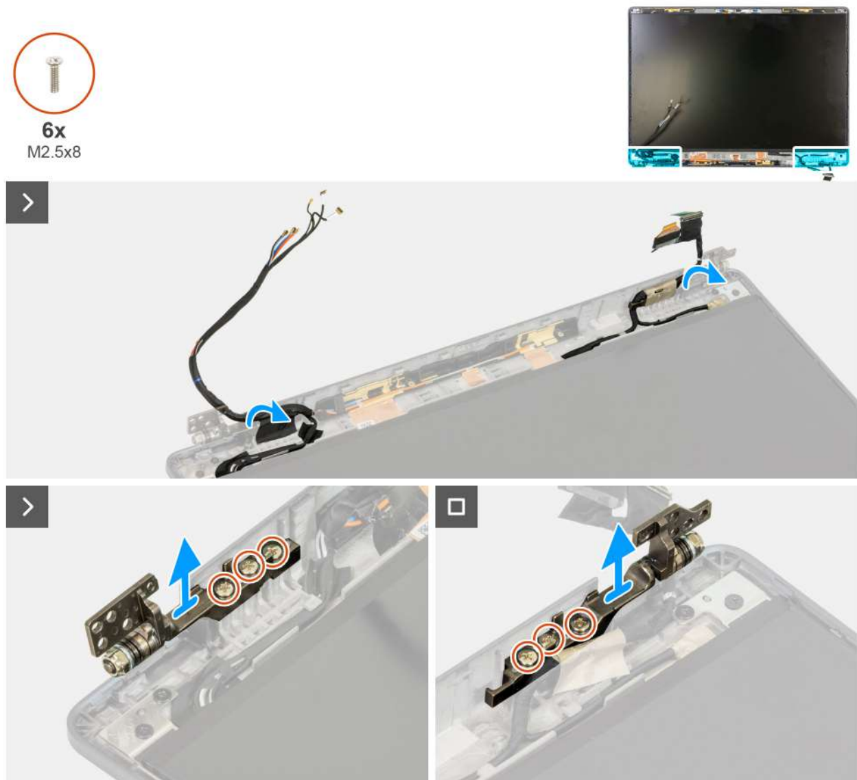
Figure 99. Removing the display hinges
