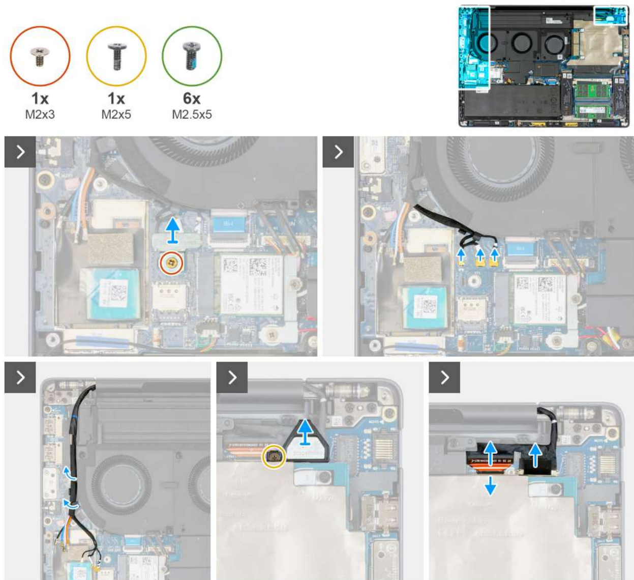
Figure 63. Removing the display assembly
