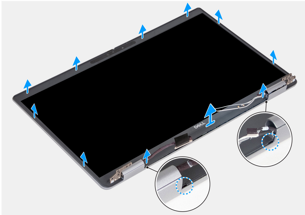
Figure 74. Removing the display bezel
