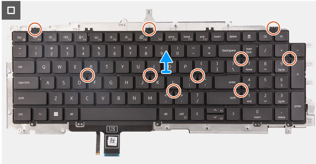
Figure 66. Removing the keyboard
